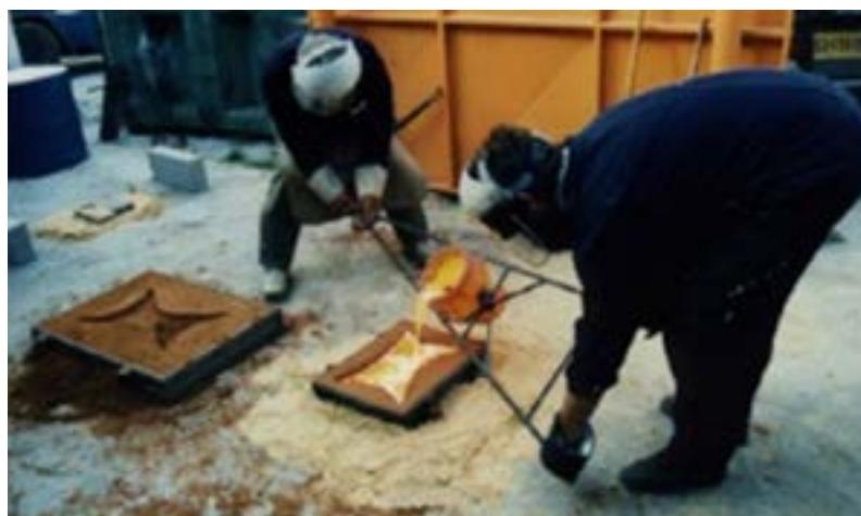
Experimental casting of molten copper in the form of an oxhide ingot. Image courtesy of V. Kassianidou.
